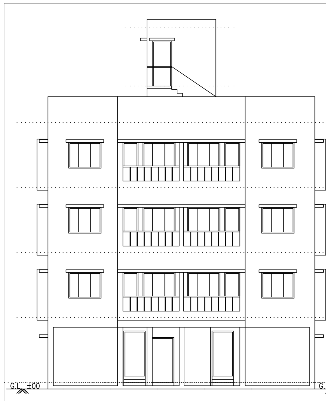
FRONT (EAST) SIDE ELEVATION SCALE=1:100
