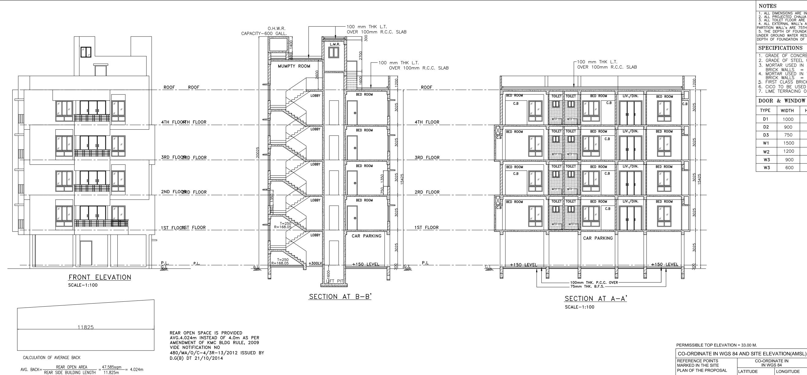
. ALL DIMENSIONS ARE IN MM 2. ALL PROJECTED CHAJJA ARE 500 WIDE. 3. ALL TOILET FLOOR ARE WATER TIGHT. 4. ALL EXTERNAL WALL'S ARE 200THK. & ALL INTERNAL PARTITION WALL'S ARE 75THK. EXCEPT OTHER WISE MENTIONED 2). 5. THE DEPTH OF FOUNDATION OF SEPTIC TANK AND SEMI UNDER GROUND WATER RESERVOIR WILL NOT EXCEED THE DEPTH OF FOUNDATION OF BUILDING. SPECIFICATIONS . GRADE OF CONCRETE USED - M20 . GRADE OF STEEL USED - Fe500 3. MORTAR USED IN 200mm & 250mm THK. BRICK WALLS = 1:6
