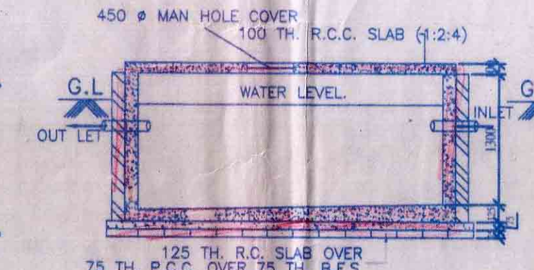
DETAIL OF S.U.G. TANK SCALE 1:50
